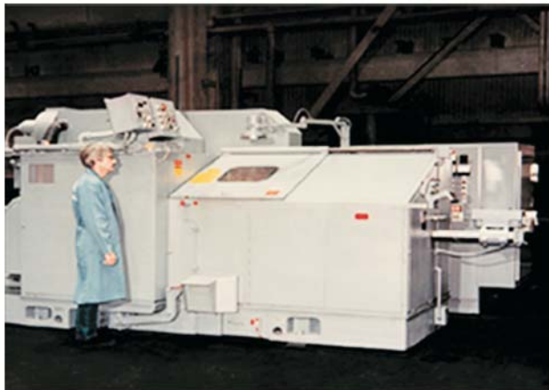
Example of 2 die & 3 punch machine
