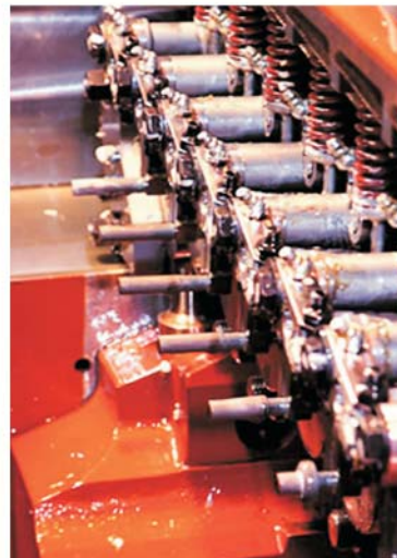
Die Area of 6 die & 6 punch Advanced FORMAX Cold Former
